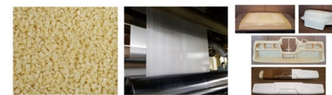
Agricultural electric vehicle parts based on cellulose nanofibers developed by Dr. Jung Yong-il's team. From left: pellets, prepreg, other parts.
